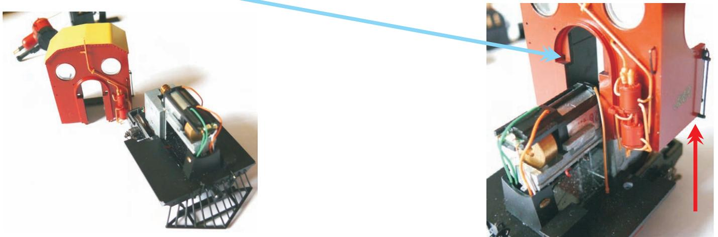
6. This disassembly allows access to both bearings on the motor for lubrication and clean contacts on the rear of the rear wheels for cleaning purposes. To gain access to the contacts on the front wheels for cleaning slide the running board forward.
